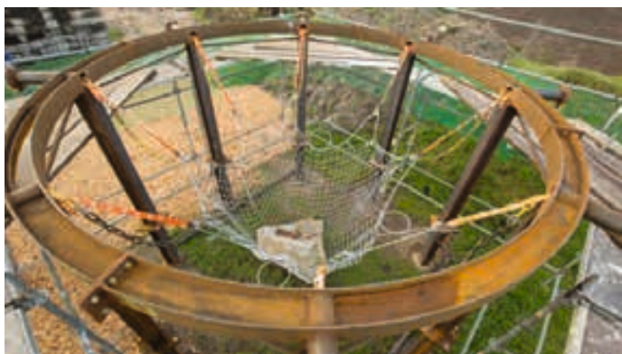
Actual condition following the drop test, with triggered „absorbers“
