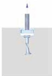
Breakout of stud under tensile loading
