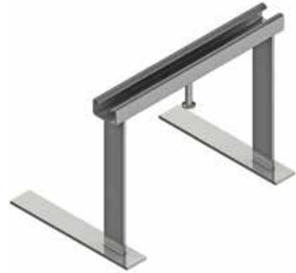
Special assembly made for connections on to edge of the slab. Channels are welded on to lugs that can have height distances to enable quick fixing on to the metal deck
