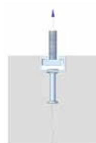
Splitting of concrete under tensile loading
