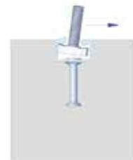
Breakout of channel lips under shear loading
