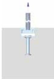
Breakout of T head bolt under tensile loading
