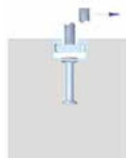
Breakout of T head bolt under shear loading
