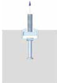
Breakout of channel lips under tensile loading
